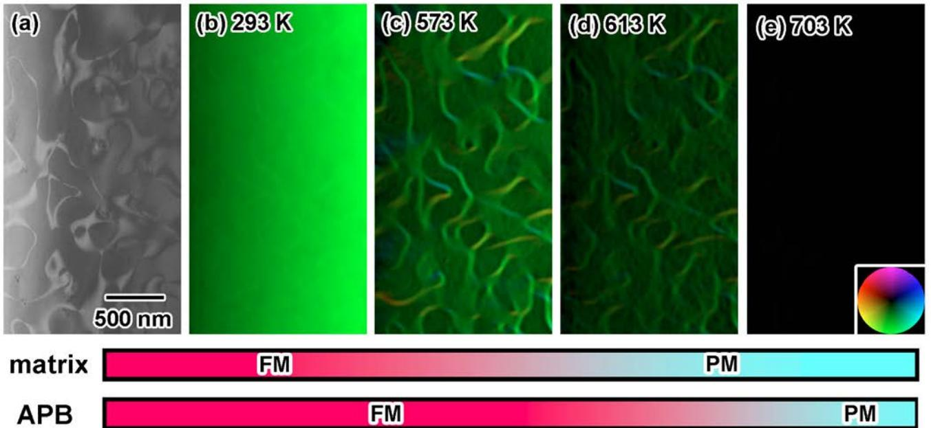
FIG. 1. Magnetic anomaly in APBs observed in  $\text{Fe}_{70}\text{Al}_{30}$ . (a) TEM image showing the locations of APBs. (b)-(e) Mapping of the phase gradient, representing the in-plane magnetic flux density. Refer to the color wheel for the direction and magnitude of the magnetic flux. FM and PM represent ferromagnetic and paramagnetic, respectively. Reprinted from Ref. 1.
